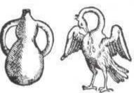
Above: the pelican, with two necks for continuous distillation, took its name from the bird.
