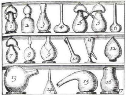
Left: apparatus that would have been used in a laboratory in the late 17th century. Although many of the vessels illustrated have since become obsolete, the following are still used in chemistry laboratories at the present time: two forms of the matrass, now called a flask, 4 and 6; the glass funnel, 14; and the retort, 16.
